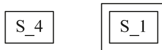
Figure 104: Steps in Sequential Function Charts: (left) general step and (right) initial step
