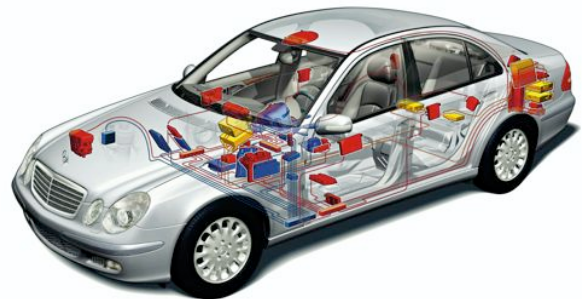
Fig. 1. ECUs and buses of Mercedes-Benz W211 vehicle. From DC-Media.
