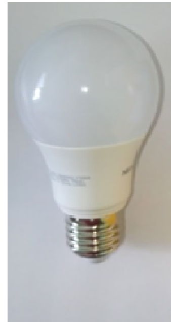
LED Lamp – Sample 7 - Neolux, 9.5W, 230V, Ra=80, 806lm, 15000h, warm light 2700K
