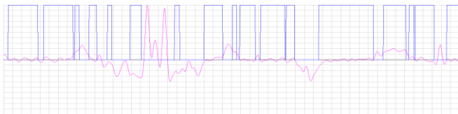
(b) Filtered curvature signal (function of contour point index [orientation in contour: left to right], violet, scaled to 1.0) and binary indicator signal for circular segments (function of contour point index [orientation in contour: left to right], blue)
