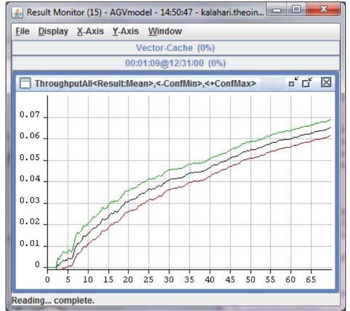
Fig. 4. Result monitor showing the transient evolution of overall throughput with confidence intervals
