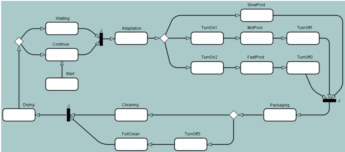
Figure 4: Operational model of the workbench.
