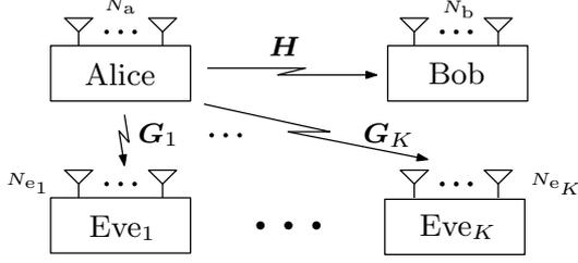
Fig. 1. MIMO Gaussian wiretap channel with  $K$  eavesdroppers.
