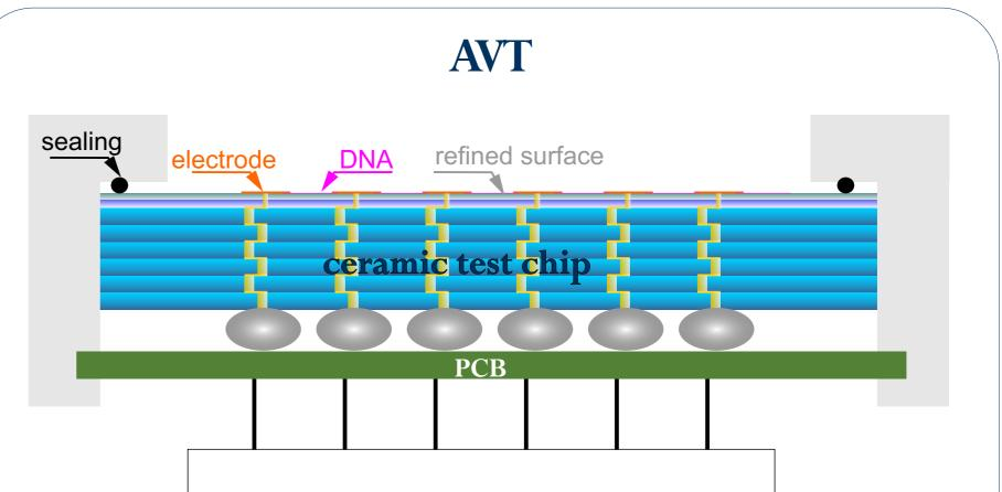
*Milestone 1:* Functionalization of large contact surfaces with oligonucleotides*Milestone 2:* Functional DNA Memristor*Milestone 3:* Switchable system through the reversible self-organized attachment of short oligonucleotides
