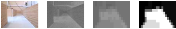
Figure 1. The steps of image preprocessing for KHEPERA: the original picture (left), the blue-yellow-activations (2nd f. left), after threefold subsampling (2nd f. right), and dynamic adaptation (right).
