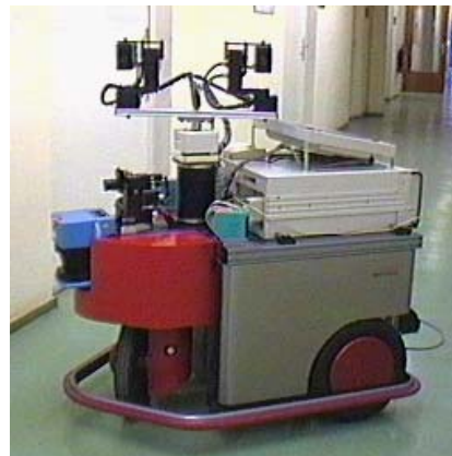
Figure 1. The mobile robot MILVA, provided with 68040-VME-system, 2 PC-systems, CNAPS-board, framegrabbers, and several sensors (3 cameras, laserscanner, ultrasound and infrared distance measures, bumpers).
