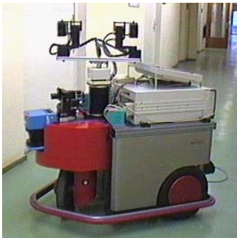
Fig. 1. The mobile robot MILVA. Provided with the necessary on-board equipment (68040-VME-system, 2 PC-systems, CNAPS-board, framegrabber) and different sensors (3 cameras, laserscanner, ultrasound and infrared distance measures, bumpers) MILVA serves as the testbed for the human-machine-interaction.
