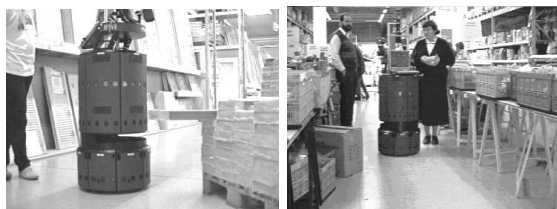
Figure 1: Our experimental platform PERSES operating in a home store, a cluttered and un-engineered environment.
