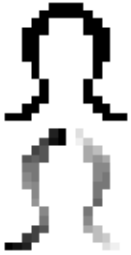
Figure 6: Illustration of the statistically determined contour model by the binary contour shape (top) and the local orientation values along the contour (bottom). Orientation angles are coded by gray values (0°: black; 90°: medium gray; 180°: white).
