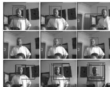
Figure 15: Person tracking experiment. The frames indicate those locations where the tracked person is most likely expected.
