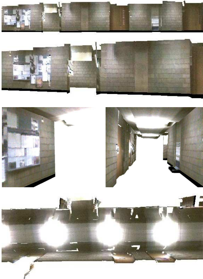
Figure 3: Views of a compact 3D texture map built in real time with an autonomously exploring robot.
