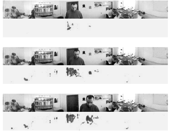
Figure 3: A few images from the beginning of a sequence are shown together with the corresponding results from the skin color classification. The intensity of the output from the skin color detector rises from the first to the last image in the sequence because of the effects of the automatic white balance.
