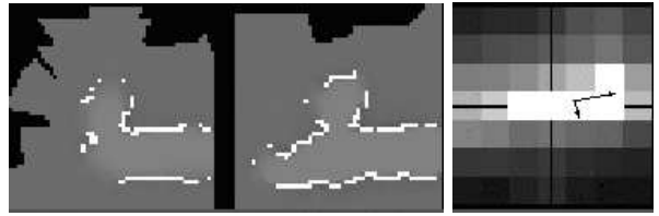
Figure 8: left: features in the temporary map, center: features in the static map, right: correlation matrix (2d, for best rotation angle d\phi , with eigenvectors highlighted)
