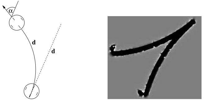
Figure 1: left: The robot drives a circular arc instead of a straight line. right: The map is distorted due to the wrong perception of the robot's own motion. Actually the environment consists of one straight corridor (black: free space, white: obstacles, grey: unexplored)
