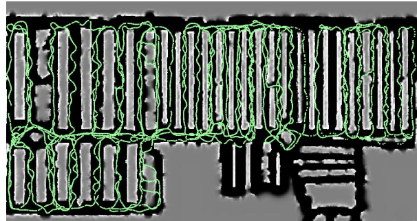
Fig. 6. An example of a grid map overlaid with a visual map. Only a part of the entire area is displayed here.
