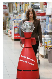
Fig. 1. Experimental platform - the interactive mobile shopping assistant TOOMAS based on a SCITOS A5 (by MetraLabs Ilmenau, Germany) during an interactive guided tour in a home store. The SonyRPU camera at the top of the robot head yields the panoramic images for the appearance-based approach presented here.
