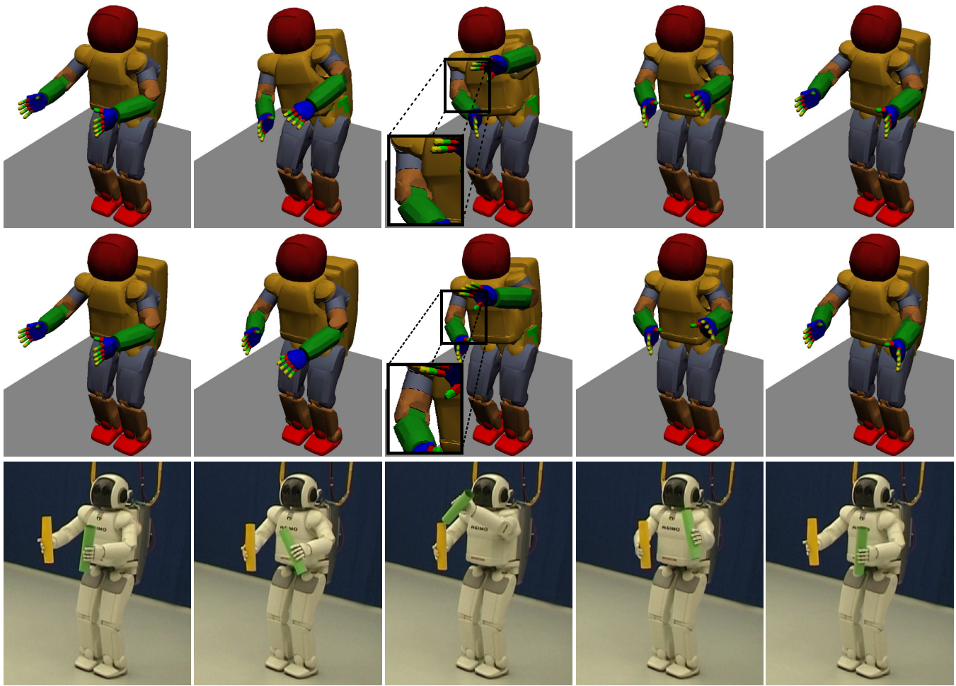
Fig. 8. Imitation of the pouring task without (top row) and with collision costs (center row). Note how the movement is optimized in order to avoid the self-collision in the middle of movement while the pouring task is still being performed. The bottom row shows the real performance of ASIMO after the movement optimization
