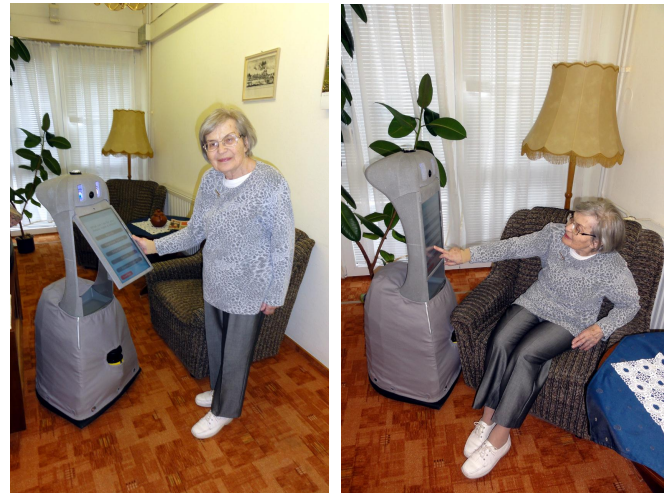
Fig. 1. 89 years old lady in interaction with the mobile home robot companion (pre-final version) developed in the CompanionAble project [1].
