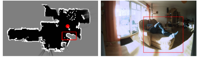
Fig. 5. Place definition. (Left) Bounding box (red rectangle) of one place (the couch) in the occupancy map of the test apartment. The robot is in its observation position (red circle). (Right) The place’s bounding box projected into the camera image shows the couch with the user resting on it.
