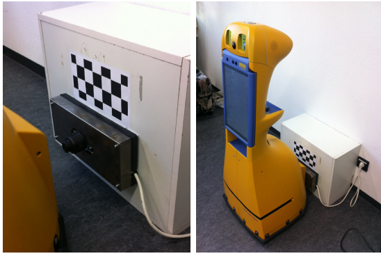
Fig. 3. (Left) Charging station with a line voltage connector inspired by the connector concept known from water boilers and synthetic markers utilized for the autonomous docking process. (Right) Robot successfully docked to the charging station.
