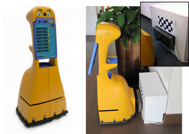
Fig. 2. Left: Scitos G3 platform developed as a companion robot for CompanionAble. Right: Robot charging and close-up of the charging station.
