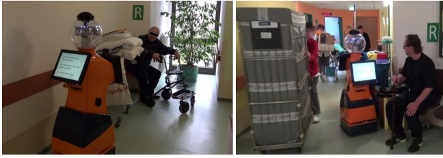
Fig. 6. Critical situations preventing successful approaching: (left) laundry trolley and own walker prevent approaching, (right) dynamic obstacles block optimal interaction position in front of the patient.
