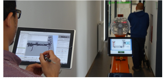
Fig. 5. Tablet-computer based correction interface for correcting lacking or wrong decisions allowing for an interruption-free testing process.
