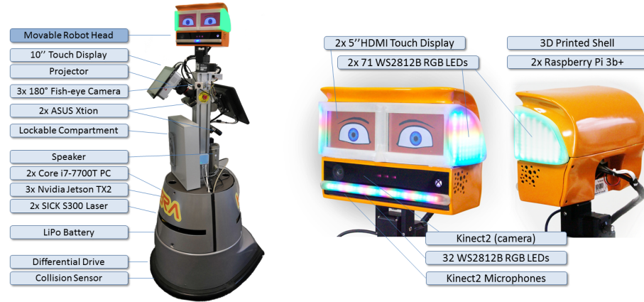
Fig. 1: Robot HERA with its sensors, interaction devices and the robot's head.
