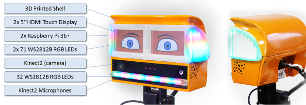
Figure 3: The robot's head with its components.
