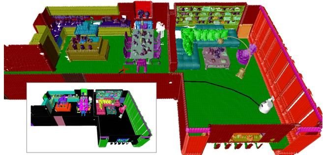
Fig. 1. Panoptic occupancy NDT (P-NDT) map built with predicted panoptic segmentation of EMSANet [4] and voxel size of 10cm for scene *ai\_051\_001* of the Hypersim [5] test split. Bottom: corresponding instance map. Best viewed in color at 300%. Black indicates *no\_instance*, see Fig. 3 for semantic colors. Panoptic is visualized by small color differences.
