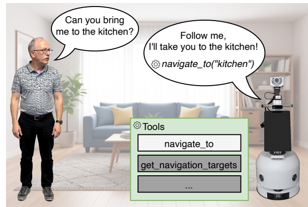
Figure 1: The proposed approach enables voice assistance for mobile robots with integrated function calling. In this example, the user's request to go to the kitchen is processed by an LLM, which triggers a corresponding tool call that the middleware executes. Because capabilities are exposed through a standardized tool interface, the same interaction pattern can be applied across different tools and robot platforms.
