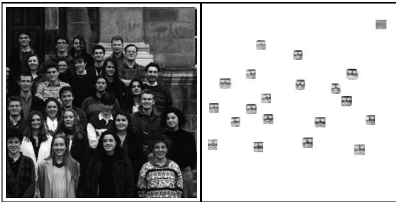
Figure 5: Detection of faces using eigenvector masks. The detected faces are marked in the right image (likelihood higher than 0.7).
