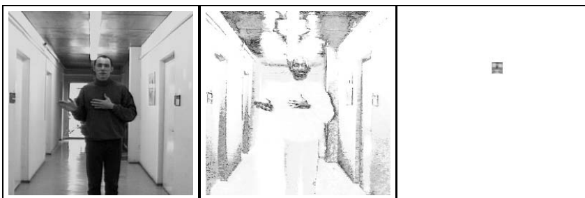
Figure 6: Skin color (middle) and face structure (right) hypotheses obtained from the input image (left), adapted by the method proposed in [8]; the used GNG consists of 49 nodes
