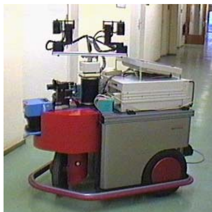
Figure 1: Our mobile robot MILVA. Provided with highly developed on-board equipment (68040-VME-system, 2 PC-systems, CNAPS-board, framegrabber) and different sensors (3 cameras, laserscanner, ultrasound and infrared distance measures, bumpers) MILVA serves as the testbed for the gesture-based interaction with a user.
