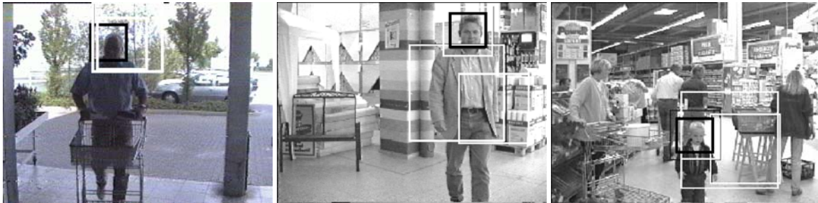
Figure 14: Typical verification results for different situations in the home improvement store. The size of the frames corresponds to the respective level of the scale space, small frames correspond to levels of high-resolution and vice versa. Final localization results, are marked as black frames. The left image shows a back light scene taken in the entrance area, where only the contour detection can provide a confident contribution for verification. In the right figure showing a crowded area in the store, the child is selected as final localization result because it is the only subject that fulfills all 3 criteria of our multi-cue approach: face and upper part of the body are oriented frontally towards the robot, skin color can be detected clearly.
