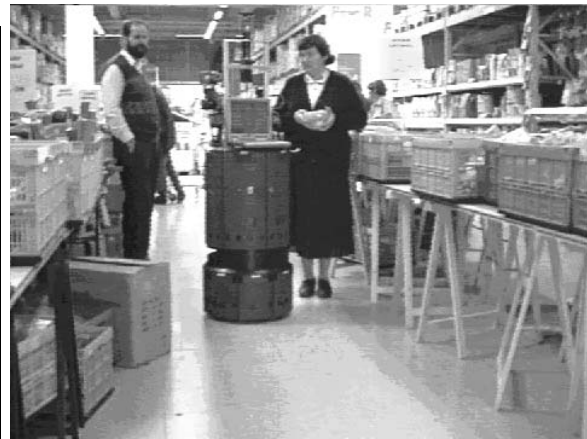
Figure 2: Left: Experimental platform PERSES. In addition to the standard equipment of two sonar and one IR-layers, PERSES is equipped with (i) an omnidirectional color camera with a 360^\circ panoramic view used for user localization and tracking, self localization and local navigation, (ii) a binocular 6 DoF active-vision head with 2 frontally aligned color cameras used for user verification and tracking, odometry correction and obstacle avoidance, and (iii) a binaural auditory system for acoustic user localization and tracking. Right: PERSES during a test run in a home improvement store, a cluttered and un-engineered environment with numerous critical obstacle configurations.
