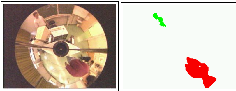
Figure 13: Motion-based segmentation of potential users in the image sequence of the omnidirectional camera. (Left) original image. (Right) segmented image, the two regions correspond with two persons at different distances to the robot.
