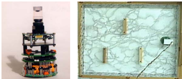
Fig. 1: Used robot platform KHEPERA equipped with an omni-directional camera (left). Top-view of the environment with the KHEPERA (right).
