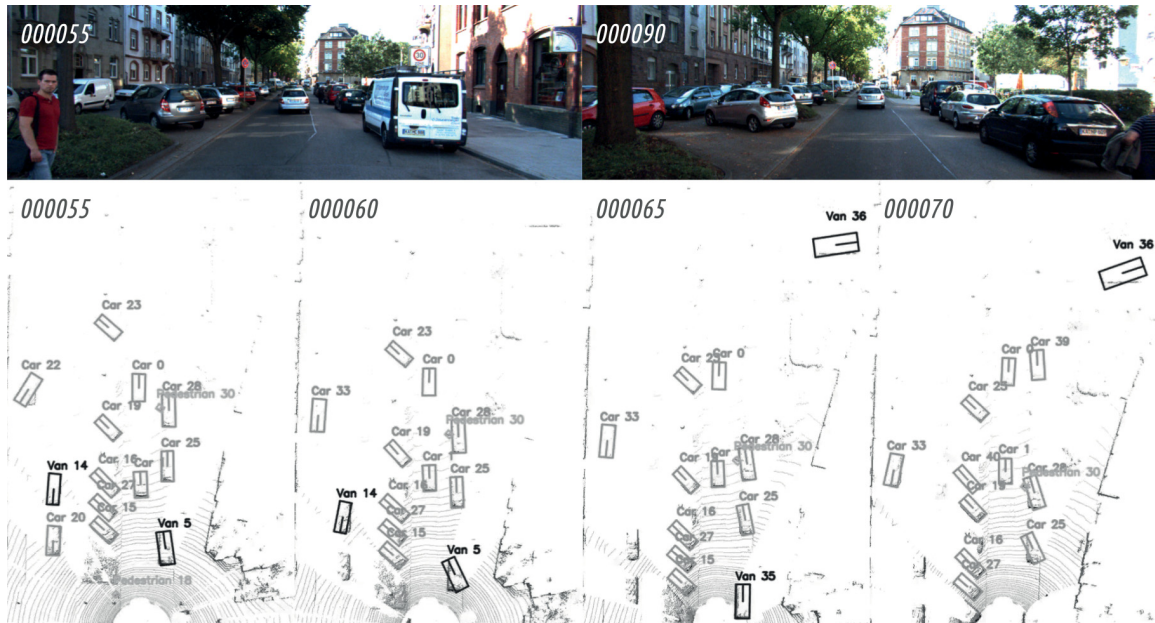
Figure 4.6: Qualitative tracking results of Complexer-YOLO on the KITTI raw sequence from 2011-09-26 number 0104 in grayscale. The figure is divided into two parts, second one (b) on the next page, to improve readability.
