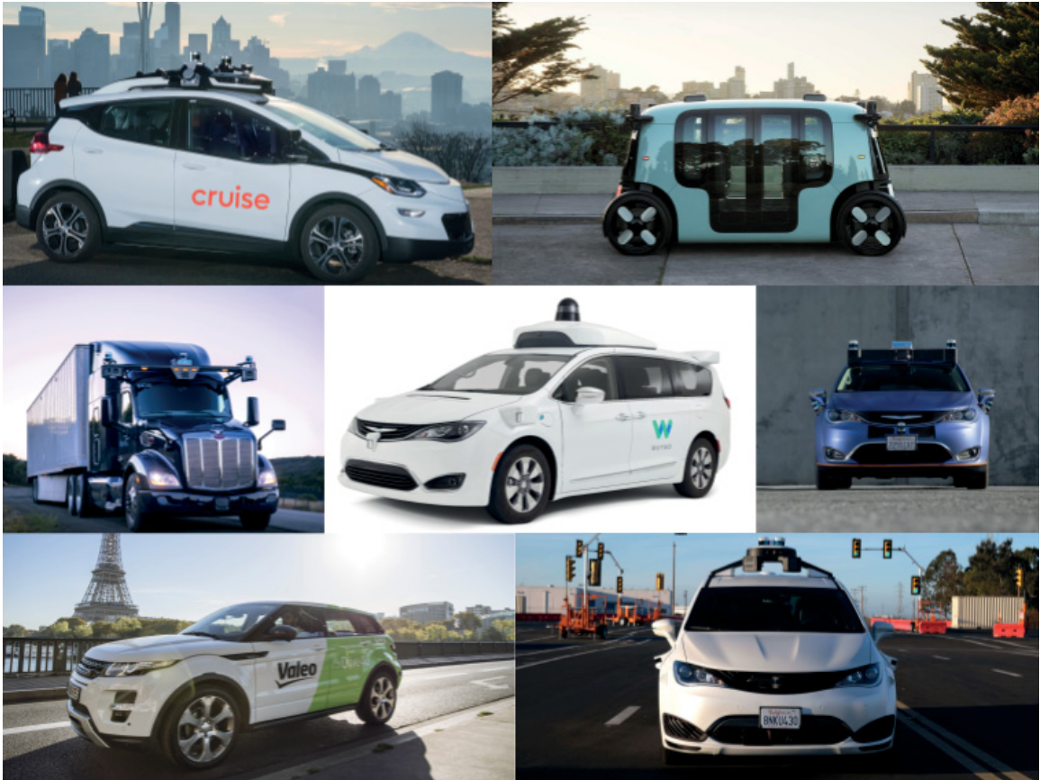
Figure 1.2: A sample collection of autonomous vehicles: All vehicles have very conspicuous sensor attachments to simplify perception except for the Valeo prototype. Images from [Cruise 2021; Zoox 2021; Waymo 2021; Aurora 2021; Valeo 2021; Level 5 2021].
