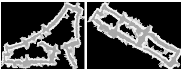
Figure 3: Results of the occupancy map building; Without (left) and with (right) vision-based correction of odometry.
