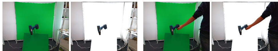
Figure 4. Example result of using the keying node in Blender on a reference recording (left) and the corresponding sample with a hand (right).
