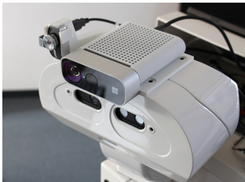
Figure 1. Cameras mounted on top of the TIAGo robot's head.
