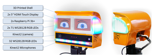
Fig. 3: The robot's head with its components.
