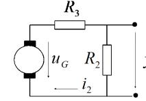
$$\Phi = \frac{N}{R_m} i_1, \quad u_G = c n \Phi = c n \frac{N}{R_m} i_1$$
