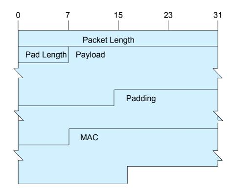
The packet format is not 32-bit-word aligned
