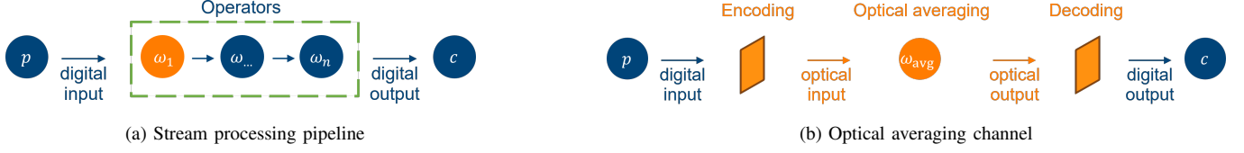
Figure 1: Mapping a stream processing operator within a pipeline to an optical averaging channel: orange parts are enabled by the optics
