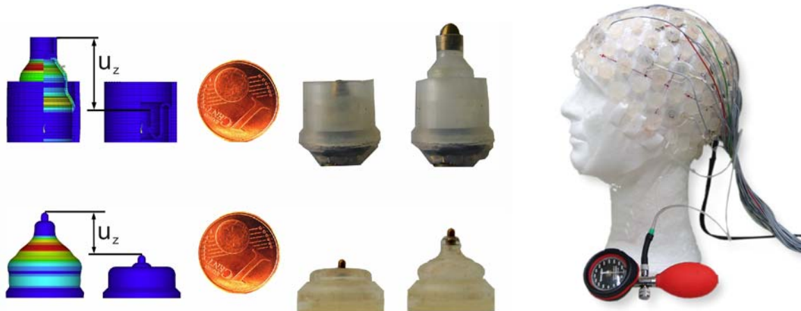
Abb.: Simulation of fluid mechanical actuators and manufactured functional models with and without internal pressure, compliant EEG cap with fluid mechanical actuators for electrode positioning
