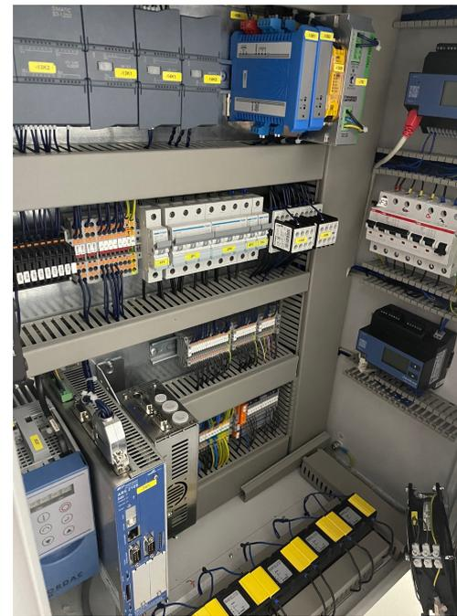
Switch cabinet of the polishing machine Stock RSP 40 with integrated power sensors.
