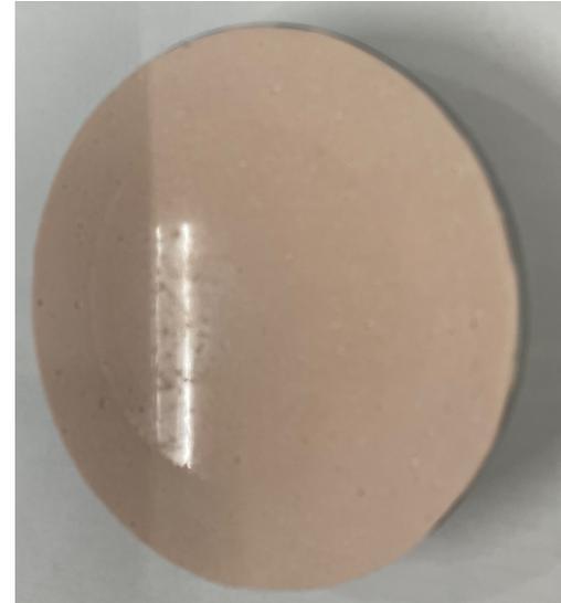
*Smearing polishing pad – the surface is smooth and reflects the light.*
