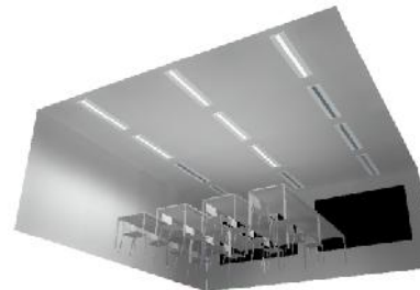
Fig.5 Lighting scene (on/off control) for period of time from 18:30 to 19:00h on a sunny spring day for a room with windows facing west
