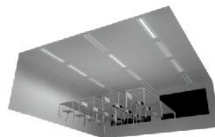
Fig.7 Lighting scene (dimming control) for period of time from 18:30 to 19:00h on a sunny spring day for a room with windows facing west
