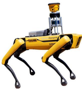
Schreitroboter SPOT (Boston Dynamics)
