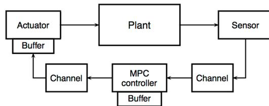
Fig. 1. Scheme of the networked control system
