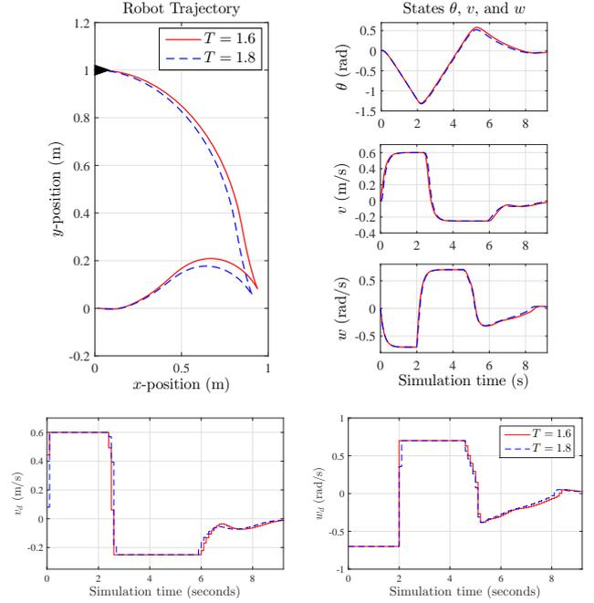
Figure 3. MPC closed-loop trajectories and controls for horizons  $T = 1.6$  (s) (red; Algorithm 2) and  $T = 1.8$  (s) (blue; Algorithm 1) with  $\mathbf{x}^0 = (0, 1, 0, 0, 0)^\top$  and  $\tau = 0.1$  (s).
