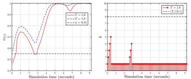
Figure 4. Evolution of the performance index along the MPC closed loop for  $\mathbf{x}^0 = (0, 1, 0, 0, 0)^\top$ ,  $\delta = 0.1$  (s), and  $T = 1.6$  (s) (solid red line; Algorithm 2) and  $T = 1.8$  (s) (blue dashed line; Algorithm 1). In addition, the evolution of the index  $k$  used in Algorithm 2 is shown (right).
