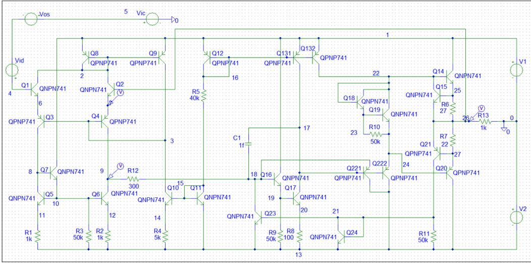
Fig. 1. Circuit diagram of an operational amplifier 741 with the typical Miller precompensation with  $C_1 = 1$  fF.
