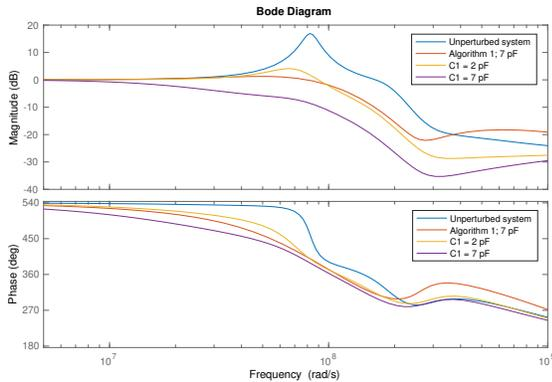
Fig. 2. The Bode diagram of the unperturbed operational amplifier shown in Figure 1, after the application of Algorithm 1 and with the standard Miller compensation with different capacitances.
