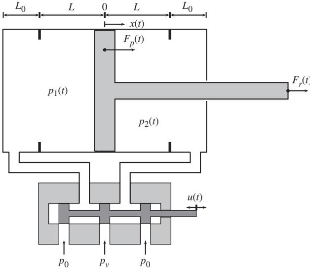
Figure 1. The pneumatic cylinder.
