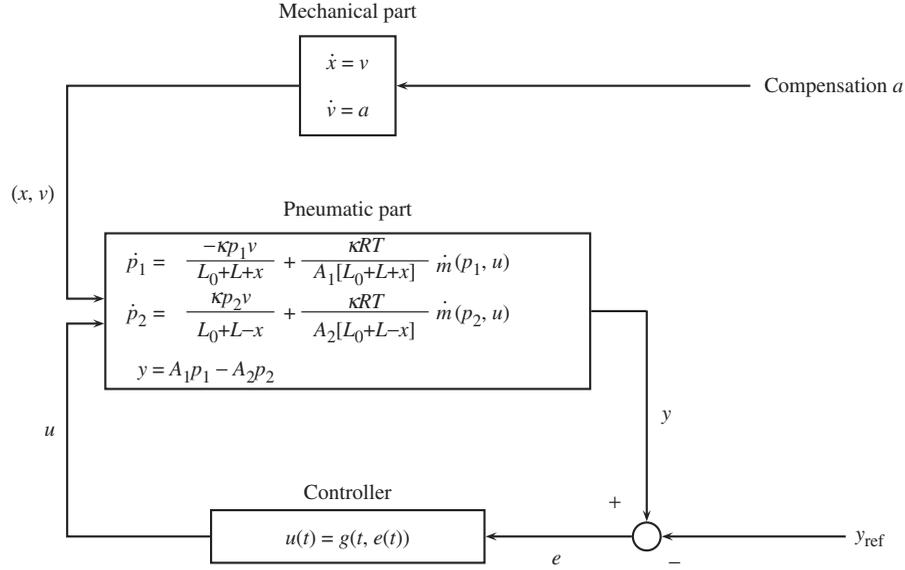
Figure 4. The model of the piston control.
