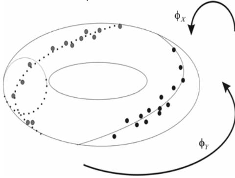
Fig. 1. Scatterplot of phase samples. The first sample  $\phi_X$  is mapped on the smaller circumference and the second sample  $\phi_Y$  is mapped on the larger one; the fitting coil is mapped as curve and dotted if behind the torus; dots behind the torus are in gray
