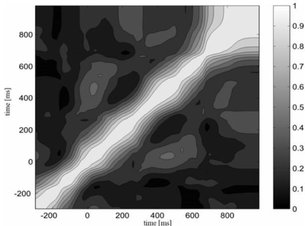
Fig. 5. Auto-correlation matrix of channel C3; with same time and sample length like in simulation
