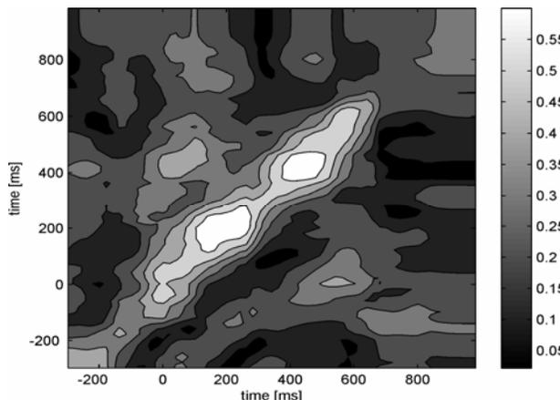
Fig. 6. Cross-correlation matrix of channel C3 and channel F4; where F4 is mapped by horizontal time; C3 is mapped by vertical time
