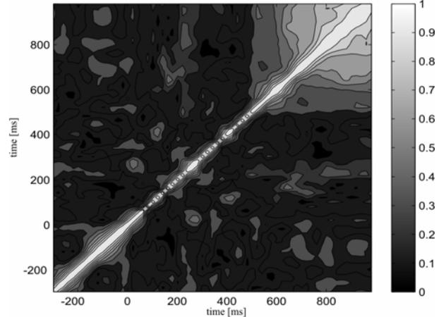
Fig. 3. Auto-correlation matrix of a simulated channel. The prestimulus interval amounts 300 ms and the poststimulus interval 1000 ms. 40 trials are realized (sample length)
