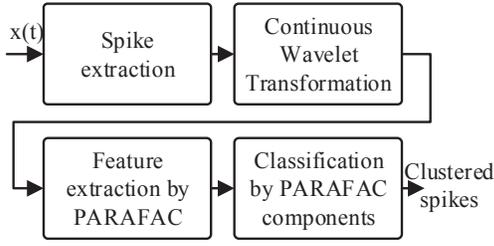
Figure 1: Block diagram of spike sorting using PARAFAC
