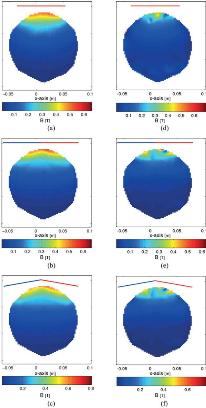
Fig. 5. Comparison of magnetic flux density in the human brain (coronal cross section). The results on the left are obtained via analytical expressions for the (a) circular, (b) 8-coil, and (c) butterfly coil, while the results on the right are obtained via proposed model for the (d) circular, (e) 8-coil, and (f) butterfly coil.
