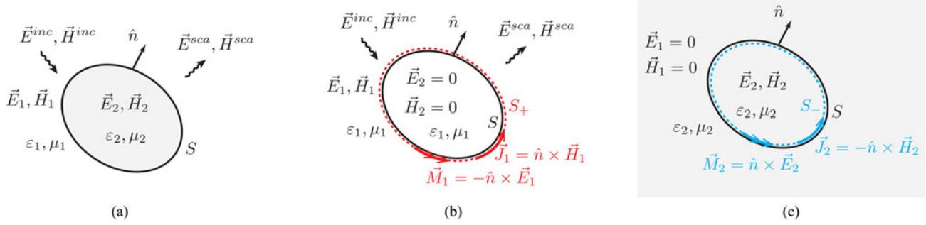
Fig. 1. Human brain as a lossy homogeneous dielectric ( $\varepsilon_2, \mu_2$ ) placed in the incident field ( $\vec{E}^{iinc}, \vec{H}^{iinc}$ ) of a TMS coil. (a) Original problem, (b) Equivalent problem for region 1. (c) Equivalent problem for region 2.
