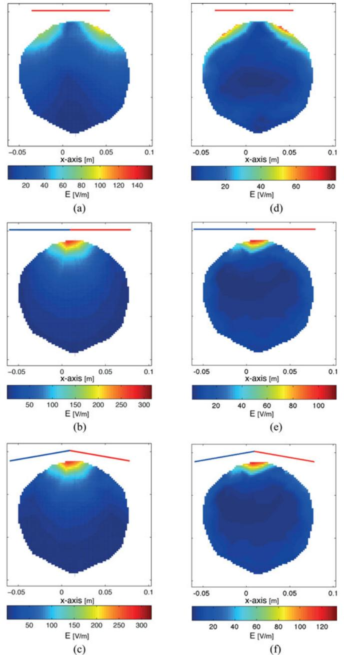
Fig. 3. Comparison of induced electric field in the human brain (coronal cross section). The results on the left are obtained via analytical expressions for the (a) circular, (b) 8-coil, and (c) butterfly coil, while the results on the right are obtained via proposed model for the (d) circular, (e) 8-coil, and (f) butterfly coil.
