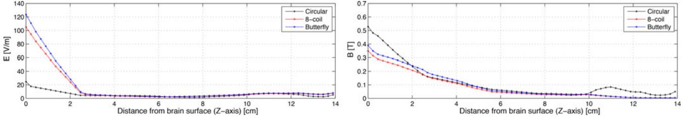
Fig. 7. Dependence of induced electric field  $E$  and magnetic flux density  $B$  on the distance from the brain surface. The values given are on the points directly under the coil geometric center.
