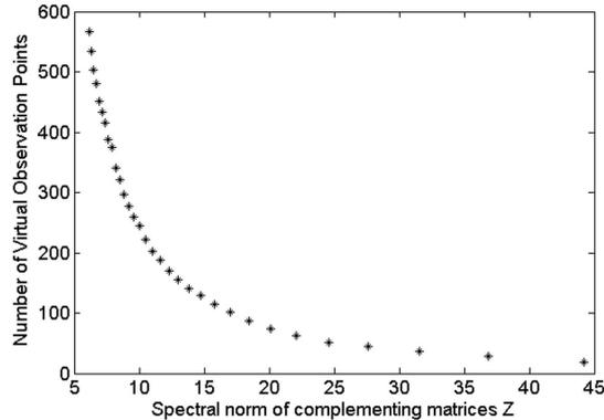
Figure 6: Number of virtual observation points  $N$  for different chosen upper limits  $u$  for the allowed maximum overestimation of the local SAR, i.e. the spectral norm of the complementing matrices  $\|Z^k\|$ .
