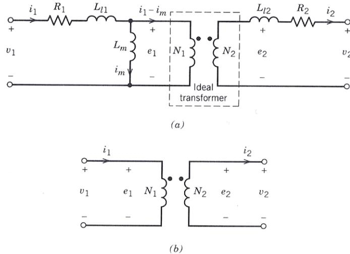
**Fig. 2: (a) Equivalent circuit for a non-ideal transformer with a lossless core and no hysteresis. (b) Equivalent circuit for an ideal transformer.**
