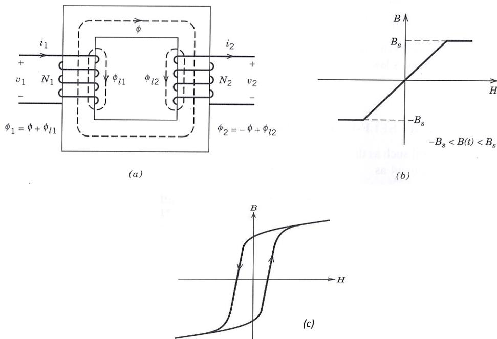
**Fig. 1: (a) cross section of a transformer. (b) Ideal  $B$ - $H$  characteristics of the core. (c)  $B$ - $H$  characteristics of the core with hysteresis.**
