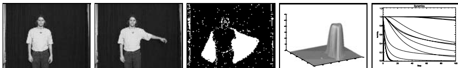
Figure 3: Demonstration of the functioning of the LRWTA. From left to right: initial and final image of a sequence, BMR image from the sequence, result of the first step of the competition/cooperation task (largest region was selected, others are temporary suppressed), time courses of the activities of all neurons until the selection of the largest region was finished.
