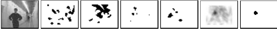
Figure 2: These pictures illustrate the localization results in an indoor environment of one pyramidal plane ( 48 \times 36 pixels). From left to right: input image, orientation filtering ( 0^\circ , 45^\circ , 90^\circ and 135^\circ ), filter arrangement result, selection within a 3D field of dynamic neurons.
